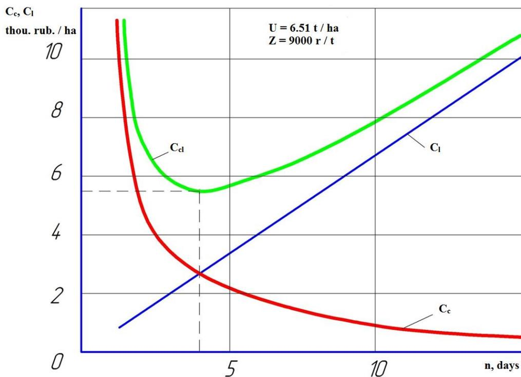
**Figure 2: Dependence on the costs of harvesting grain and crop losses from the harvesting time**
